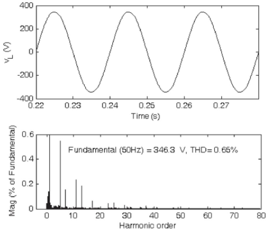
Load voltage and harmonic spectrum during the disturbance.
