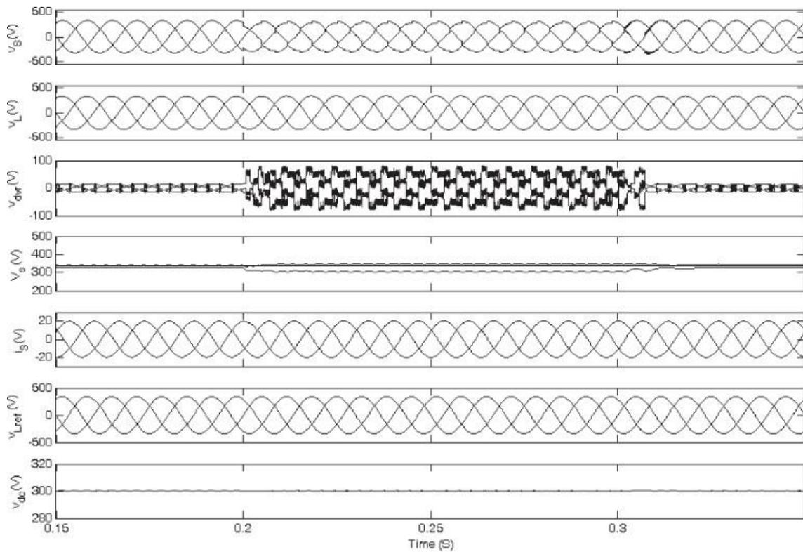
Dynamic performance of DVR during harmonics in supply voltage applied to critical load.
