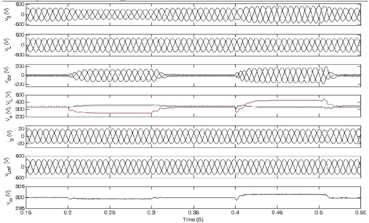
Dynamic performance of DVR with in-phase injection during voltage sag and swell applied to critical load.
