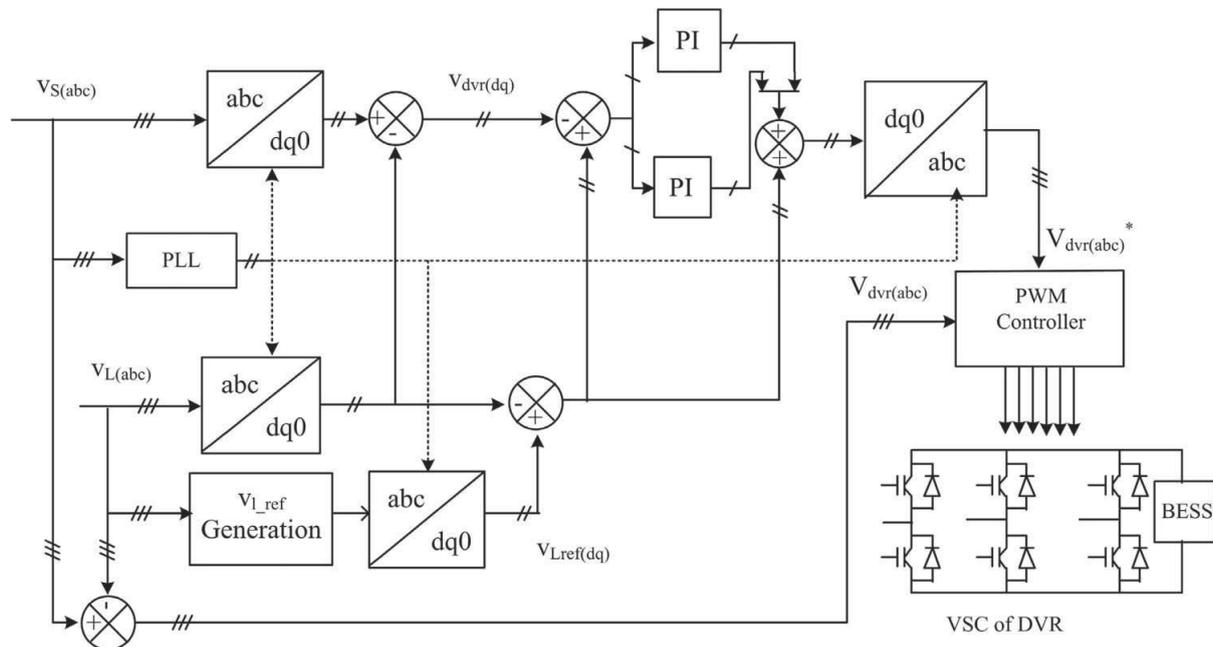
Basic circuit of DVR. (b) Phasor diagram of the DVR voltage injection schemes.
