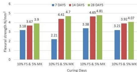
Increase in strength of various concrete mixtures over the plain concrete is also tabulated in the table 5. There is considerable increase in the flexural strength of concrete with the inclusion of foundry sand.
