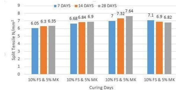
There is a considerable improvement in the split tensile strength of concrete with inclusion and increase the percentage of waste foundry sand up to 40%. It is observed that the split tensile strength increased with increasing age of curing. The maximum strength was achieved with 40% of foundry sand.
