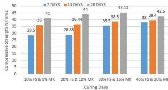
There is a considerable improvement in the compressive strength of concrete with inclusion and increase in the percentage of waste foundry sand up to 40%. It is observed that the compressive strength increased with increasing age of curing. The maximum compressive strength was achieved by 40% replacement fine aggregate with foundry sand.
