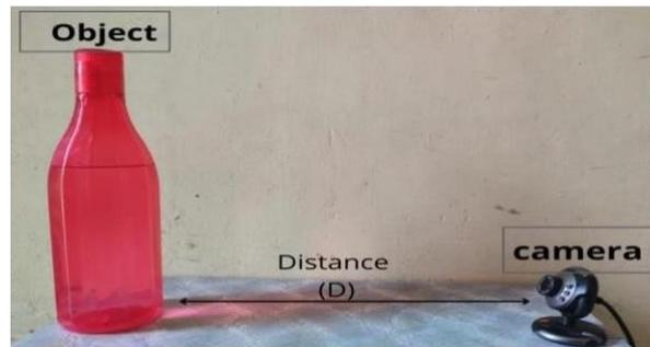
The figure 4 shows the real-time setup on distance calculation method. After determining the focal length, I can determine the distance of object to camera. If we change the distance of camera from object, the object width will also change. And through automatic image processing the perceived width of object in pixels is also changes. Thus, we get distance of object to camera. The figure 5 shows the calculated distance in “cm” unit of detected object.
