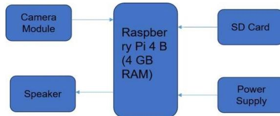
Raspberry pi 4B model of 4GB variant is connected with power supply of 5V, 3A adaptor. Camera module is connected to CSI port of raspberry pi 4B model which capture the video feed data and send to model. The data of video feed is stored in micro-SD card which is inserted in raspberry pi model. And speaker is connected to module for an audio output.
