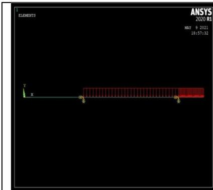
Fig No 2: Simply supported beam with UDL.
