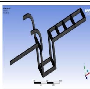
**Fig no 8: Meshing of chassis**
