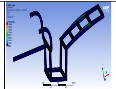
**Fig no 10: Von-Mises analysis of chassis**
