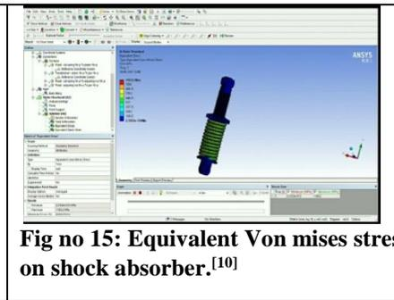
Hence, from figure no. 13 and figure no. 15, it is proven that both the actual shear stress and actual spring rate are less than the maximum values. And thus the design is considered to be safe.
