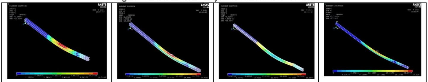
Fig no 6: Von-Mises stress analysis for various cross sections
