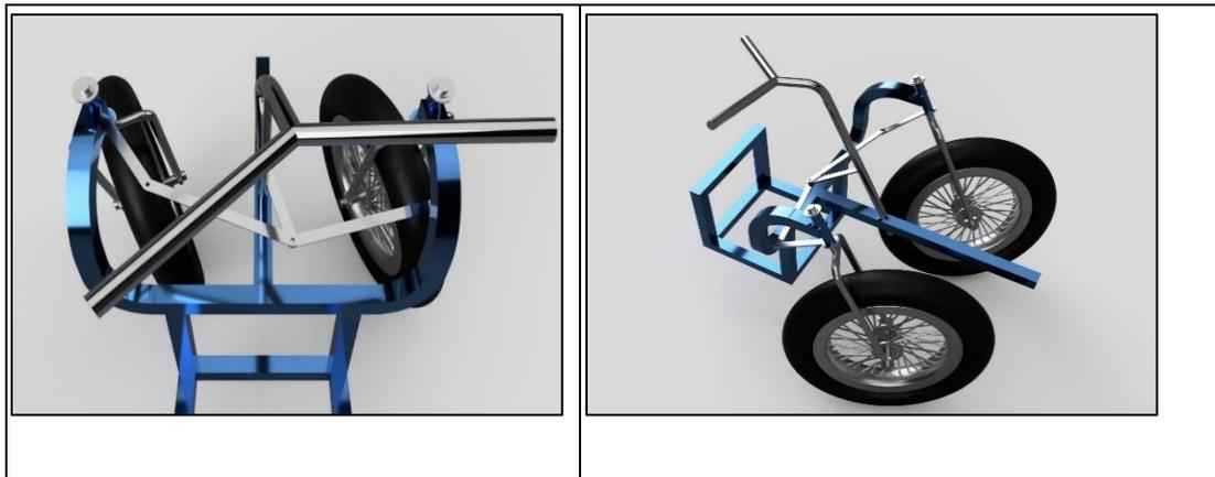
Fig no 11: CAD Model of steering system
