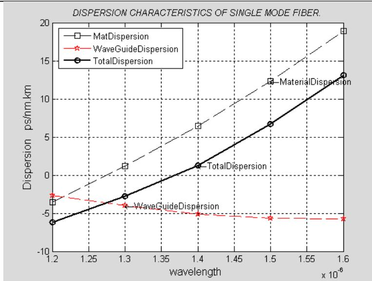
**Figure 3** - Dispersion characteristics for singlemode fiber
