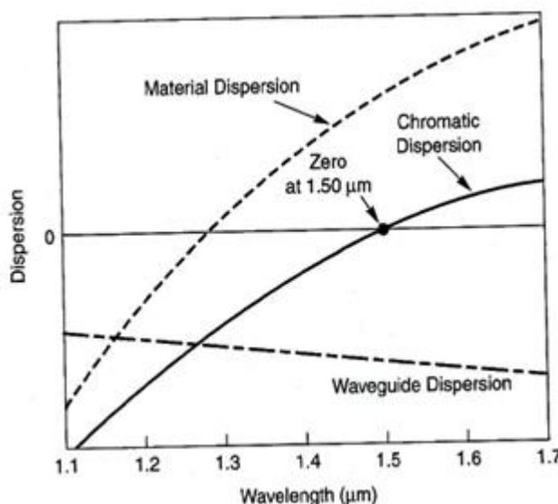
**Figure 2-** Combine waveguide and material dispersion.
