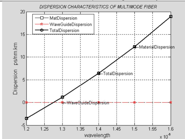
**Figure 4-** Dispersion characteristics for multimode fiber
