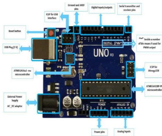
**Figure no 7:** Microcontroller (Arduino) used for controlling
