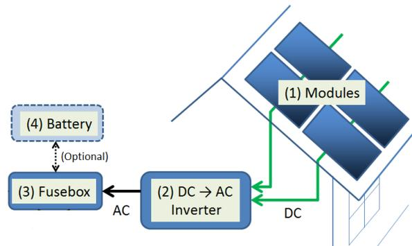
**Figure no 3:** PV system and storage of solar energy
