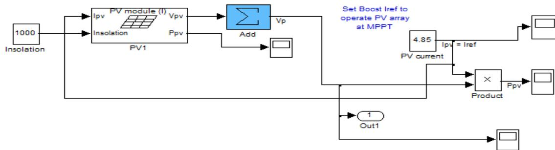
Fig.3.2: Solar model for TIBC
