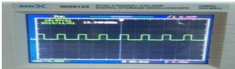
Fig.4.3: Switching Pulse for ILBC
