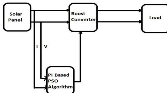
Figure 4: Block diagram
