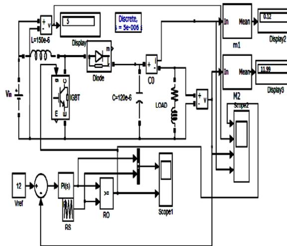
Figure 7: Simulation diagram for boost converter with PI controller
