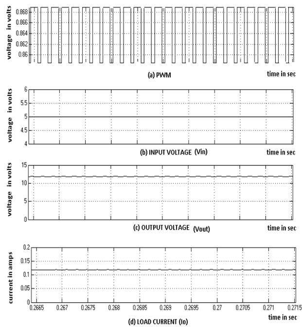
Figure 9: Simulation results for boost converter with PI controller (a)PWM , (b)Input Voltage, (c)Output Voltage and(d)Load Current
