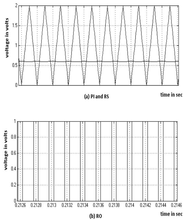
Figure 8: PWM Generation (a) PI and (b) PWM Pulses and Triangular multicarrier
