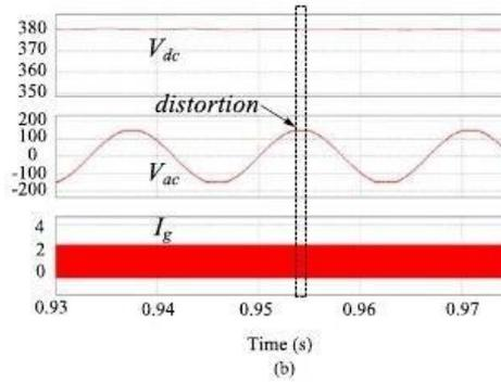
Fig. 10. Simulated waveforms of the SSBI's output voltage  $V_{ac}$ , dc-link voltage  $V_{dc}$ , and dc input source current  $I_g$ : (a) illustrating the undistorted output voltage  $V_{ac}$ , when SSBI is operated in deep DCM just above the minimum power level  $P_o > P_{o min}$  and (b) illustrating the peak-shaving distortion of the output voltage  $V_{ac}$  for  $P_o < P_{o min}$ .
