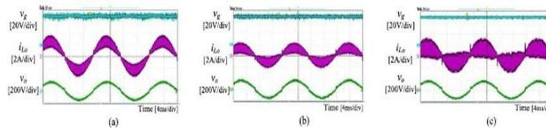
Fig 11. Experiment results of  $v_g$ ,  $i_{Lo}$ ,  $v_o$  under different output power ( $V_g = 48\text{ VDC}$ ): (a) 200W, (b) 100 W, (c) 50 W
