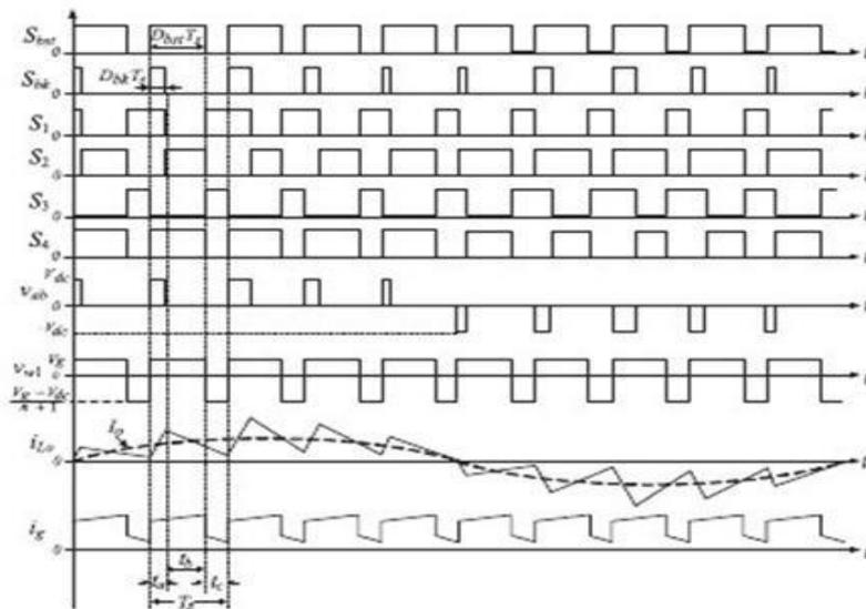
Fig 5. Key waveforms of the proposed SSBI.
