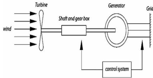
Fig.2 basic schematic diagram of wind turbine
