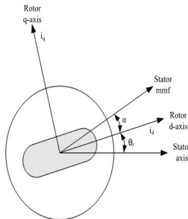
Fig 5: d-q model for the rotor reference frame
