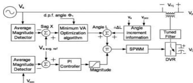
Fig. 4. Closed-loop schematic block diagram of DVR
