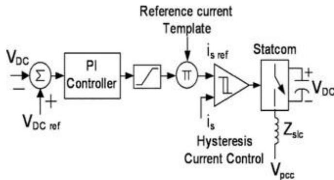
Fig.3. Closed-loop schematic block diagram of STATCOM
