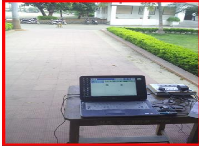
Figure 3: Experimental arrangement of motes and the Base Station for measurement of WSN parameters for outdoor deployment.
