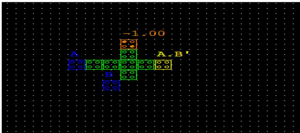
Fig. 8: Design for Boolean expression  $[(\overline{AB}) + (\overline{A + B})].A\overline{B}$  with output A.B'
