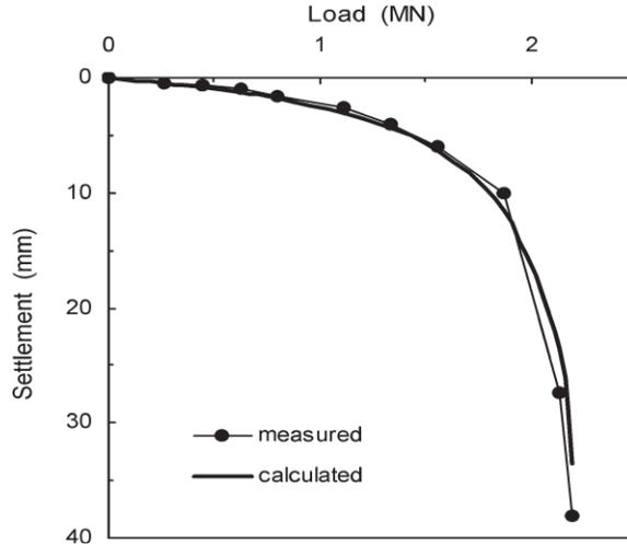
Fig. 9. Comparison of the calculated and predicted load-settlement behavior for pile groups- briaud et al. (1989)
