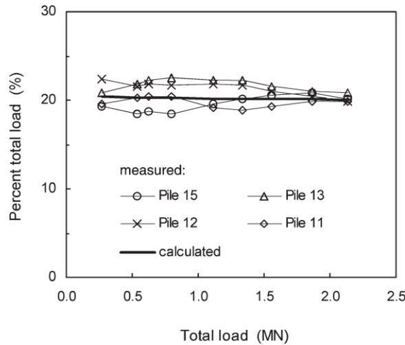
Fig. 11. Comparison of the calculated and predicted loads carried by the corner piles - briaud et al. (1989)
