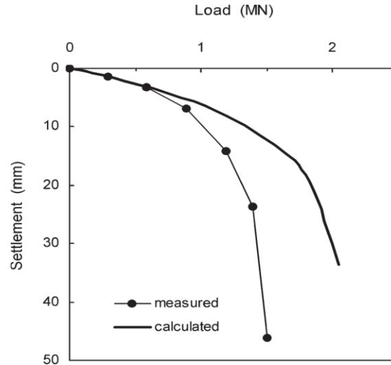
Fig. 2: Comparison of measured and predicted load-settlement behaviour for pile group-koizumi and ito (1967)
