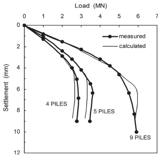
**Fig. 7:** Comparison of the calculated and predicted load-settlement behavior for pile groups- o'neill et al. (1982)
