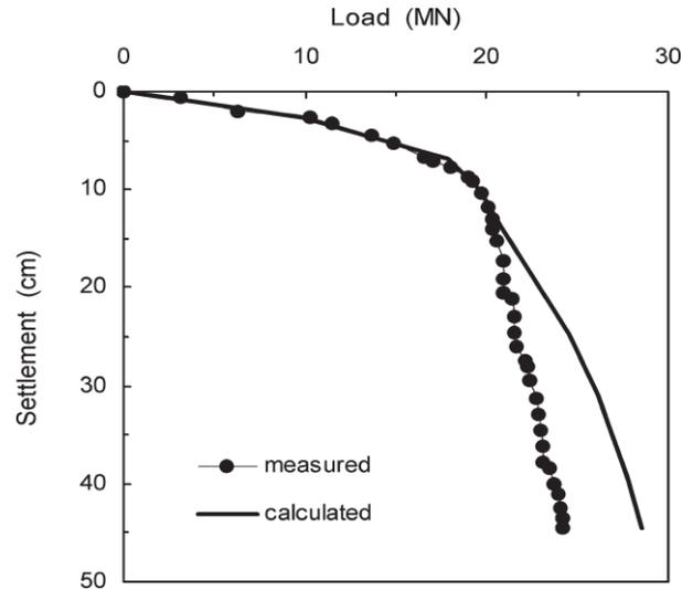
**Fig. 13.** Comparison of the calculated and measured load-settlement behavior for the pile group - conte et al. (2003)
