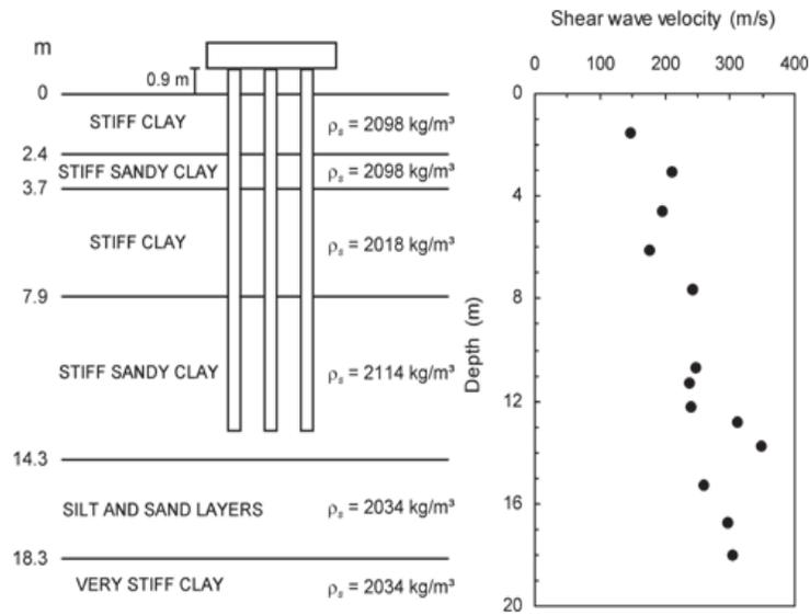
**Fig. 5:** Layout of pile group, soil profile and soil properties
