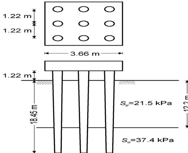
Fig. 3: Schematic diagram of pile system
