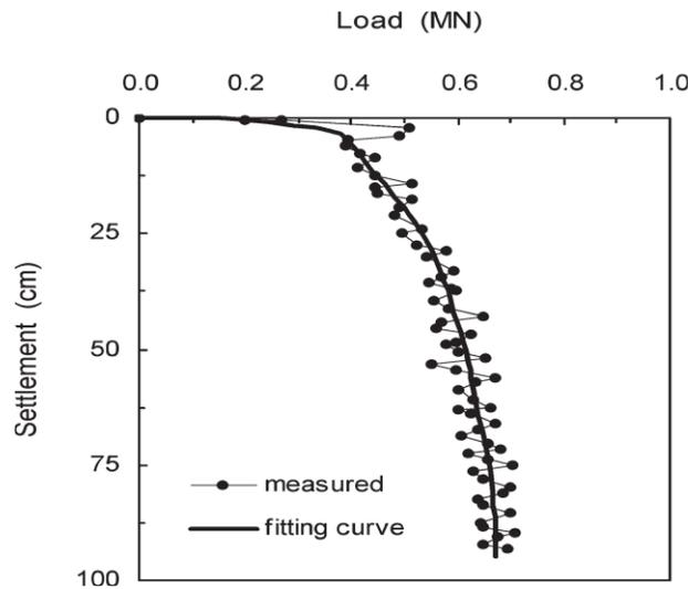
Fig. 12. Load-settlement response of single pile with indication of fitting curve - conte et al.(2003)
