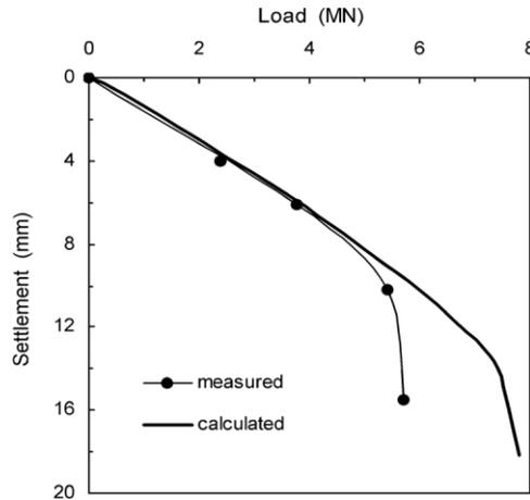
**Fig. 4:** Comparison of measured and predicted load-settlement behaviour for pile group- o'neill (1981)
