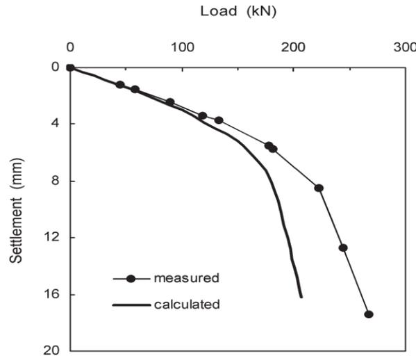
**Fig. 1:** Comparison of measured and predicted load-settlement behaviour for pile group-vesic(1967)
