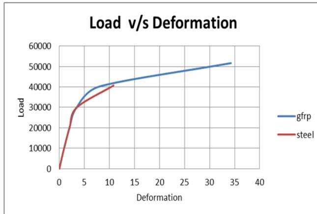
Fig no.12 Load v/s Deformation graph of Model S90 and Model G90
