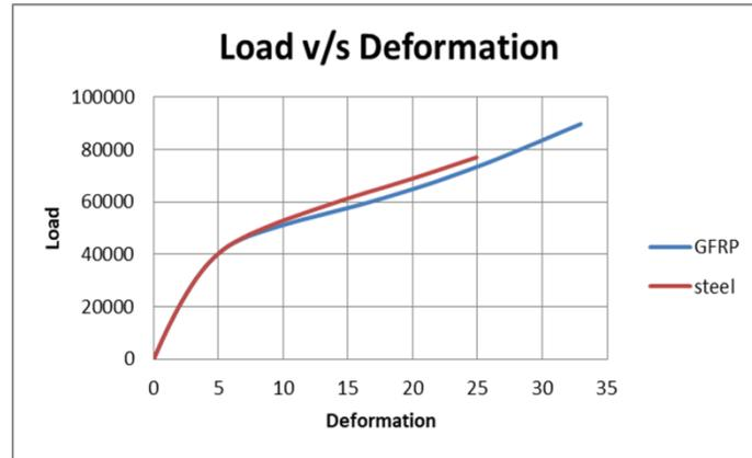
Fig no.15 Load v/s Deformation graph of Model SF90 and Model GF90
