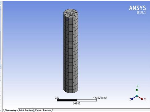
Fig no. 2 Mesh diagram of column without confinement
