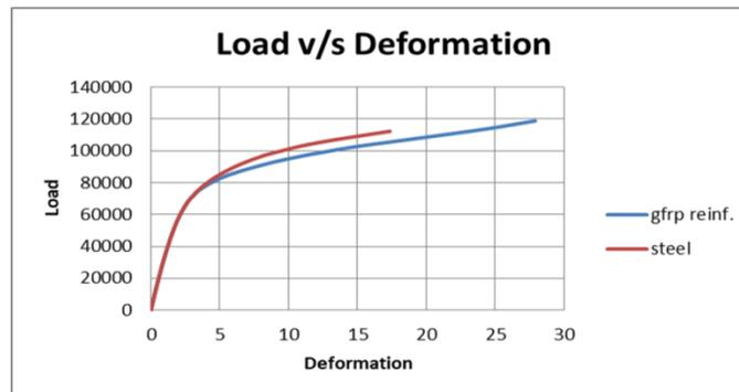
**Fig no.14** Load v/s Deformation graph of Model SF60 and Model GF60
