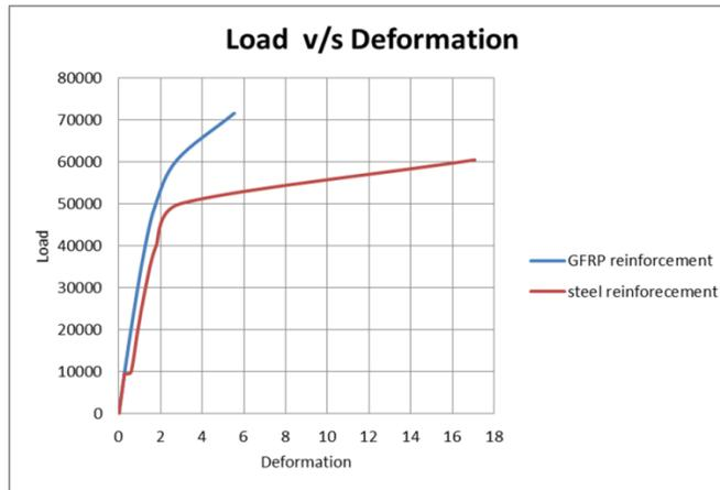
Fig no.11 Load v/s Deformation graph of Model S60 and Model G60
