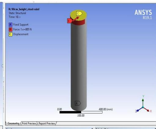
Fig no.4 Loading and support condition
