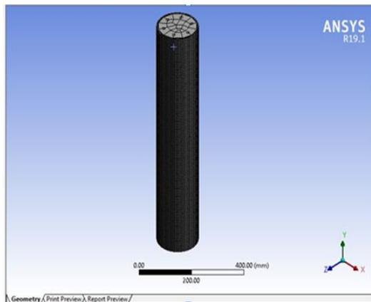
Fig no.3 Mesh diagram of column with confinement
