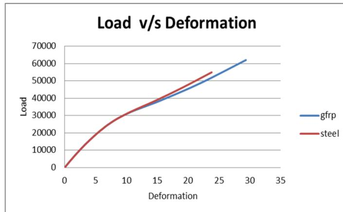
Fig no.16 Load v/s Deformation graph of Model SF120 and Model GF120
