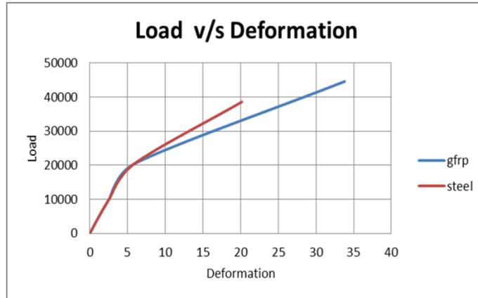
**Fig no.13** Load v/s Deformation graph of Model S120 and Model G120
