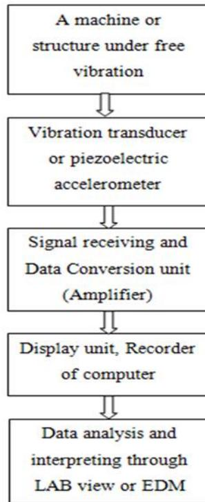
Fig.2 Block diagram of experimental modal analysis
