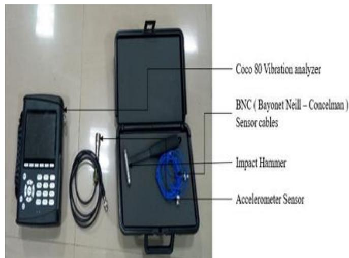
Fig.1 FFT analyzer
