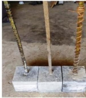
Figure 7: Specimen for reinforcement pull-out test [2]
