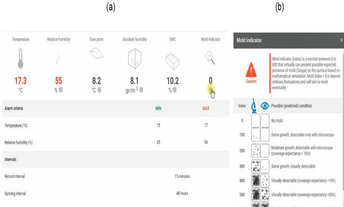
**Figure No. 10:** (a) Snapshot of Developed Platform for Monitoring Mold Growth and Alerting User, (b) Mold Growth Criteria
