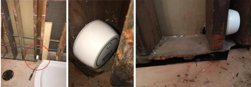
**Figure No. 9:** Deployment of SmartyLog in Damp Area for testing and validation
