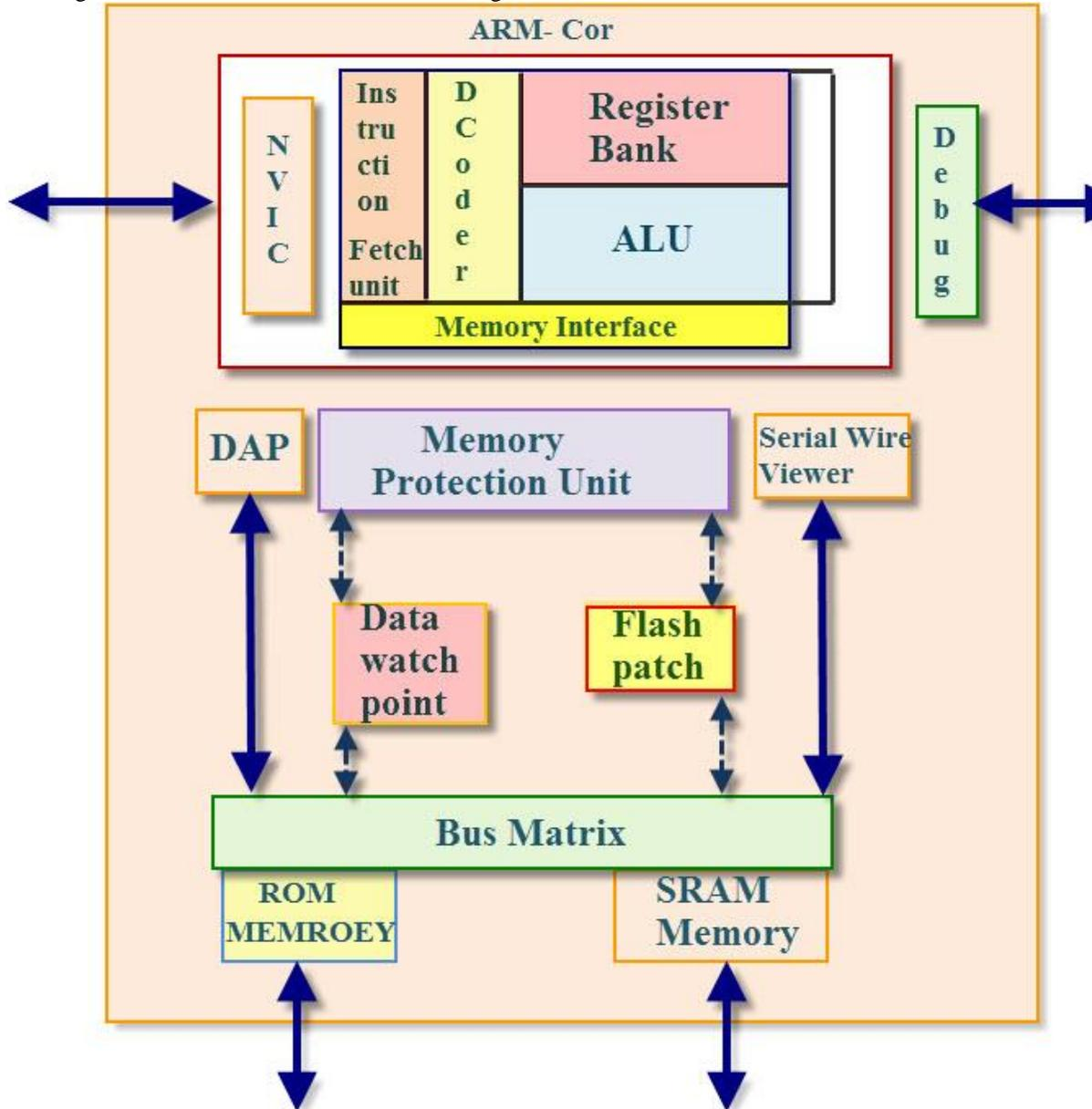
**Figure No. 3:** ARM Microcontroller Architecture
