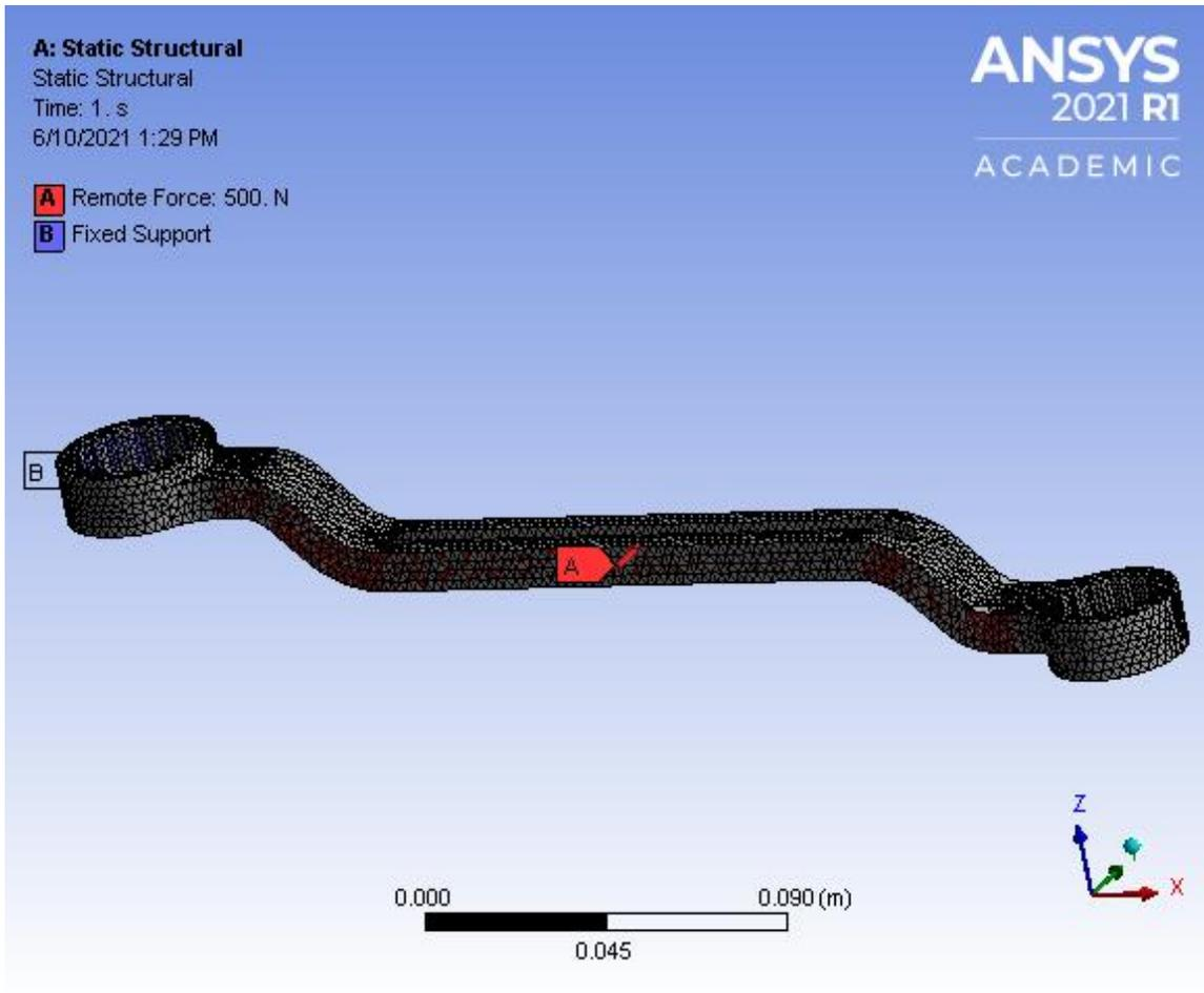
The material used for manufacturing spanner or wrench is Chromium Vanadium alloy. The structural steel is easily available, fire-resistant, and ductile. Table 2 shows the mechanical properties of the material.
