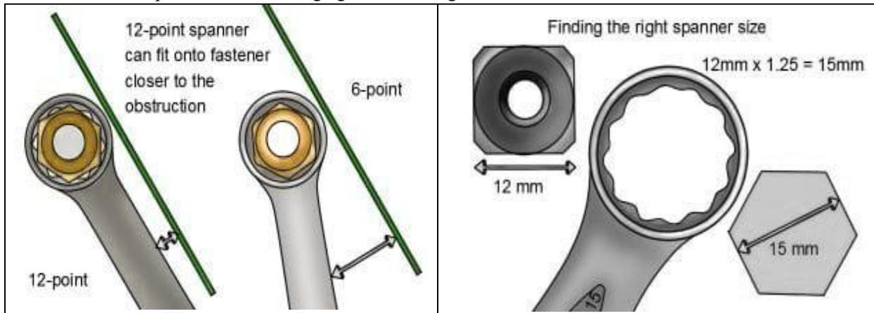
Ring spanner sizes are given as the size of a head of a hexagonal fastener the spanner can be used on. Ring spanner profile sizes are available to fit hexagonal fastener head sizes ranging from 4mm to 50mm or 5/32" to 2". The spanner length increases with the size of the spanner head, from about 100mm (4") to 500mm (19½").
