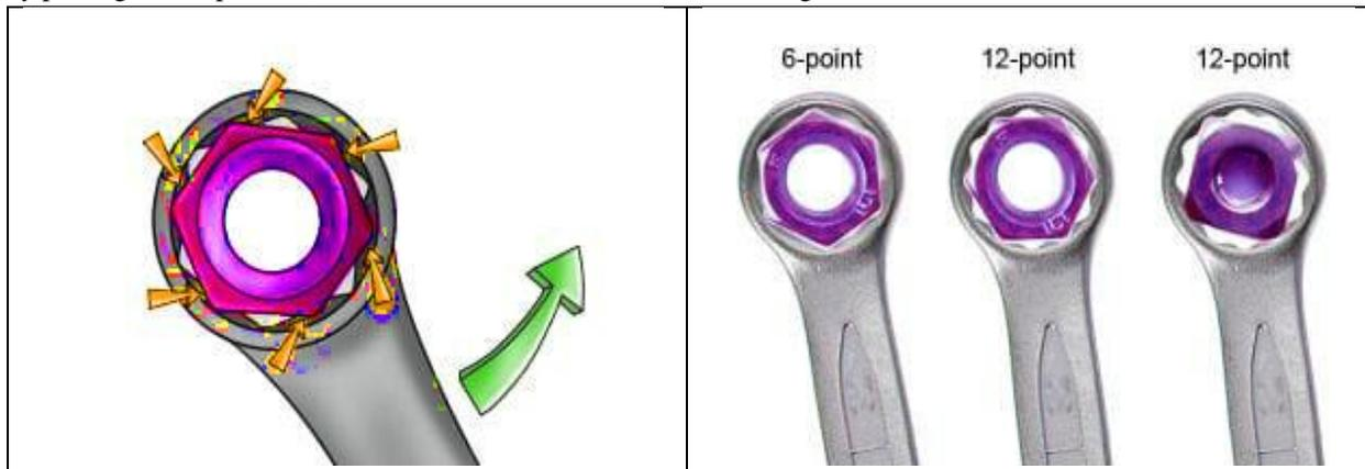
In comparison with an open-ended spanner, the ring spanners are less slippery over the fastener, because ring spanners provide large contact points with the fasteners in all possible points. This implies the turning arc will be more with large action and make the task effective and quicker.
