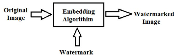
Figure 1: watermarking embedding scheme
