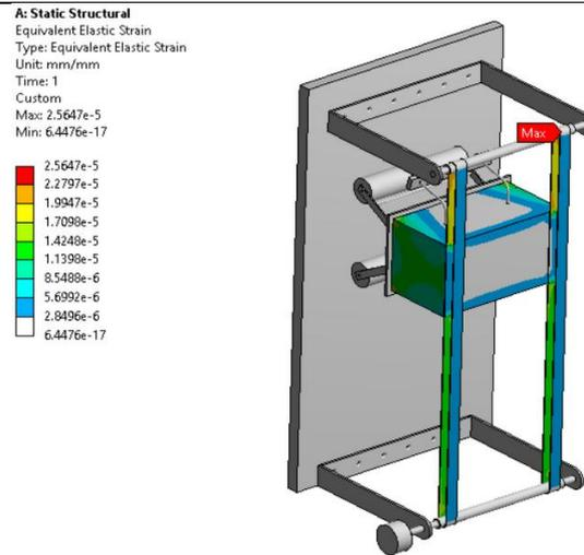
The strain induced is 25.64micron
