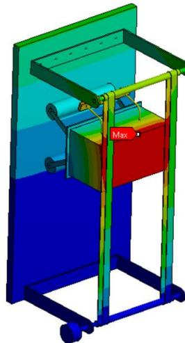
Maximum deformation induced in body is 0.013373mm
