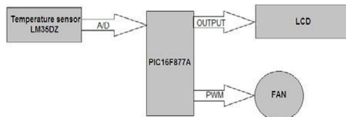
**Figure no 1:** Block diagram of fan speed control system
