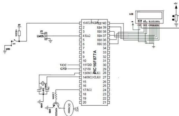
**Figure no 4:** Schematic circuit diagram of fan speed control system
