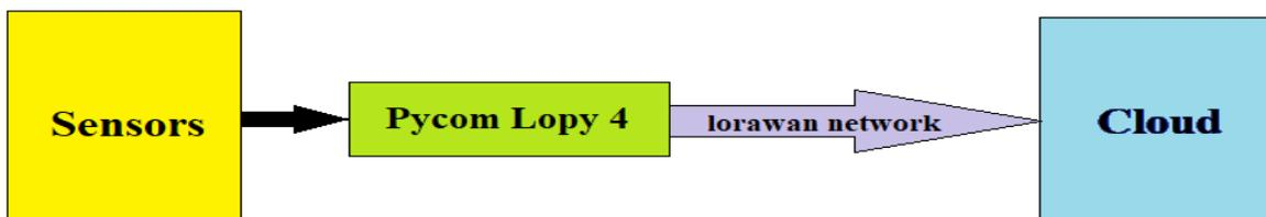
Sensors like IR sensor is connected to the Pycom Lopy 4 which process the whole received data and forward it to the cloud location through LORAWAN network.
