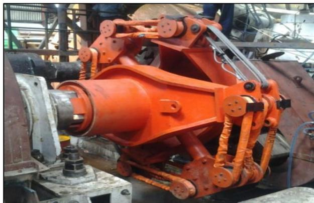
Fig. 2 Mill Rope Coupling
