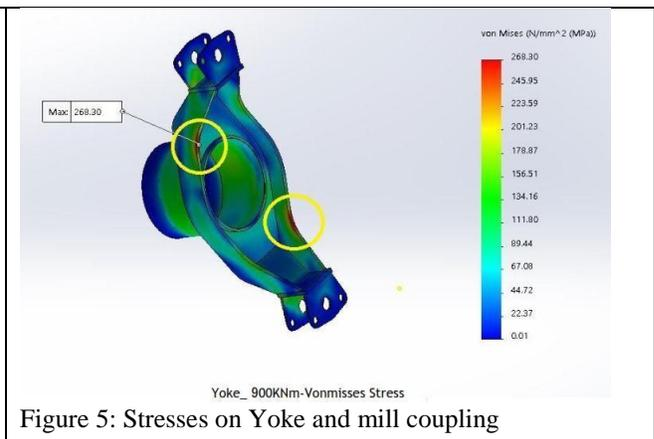
Figure 5: Stresses on Yoke and mill coupling
