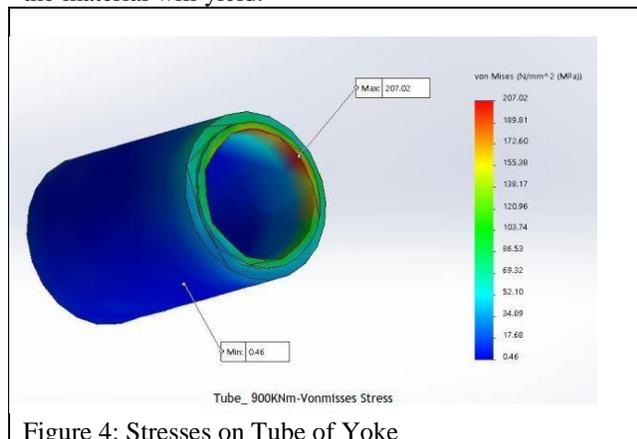
Figure 4: Stresses on Tube of Yoke
