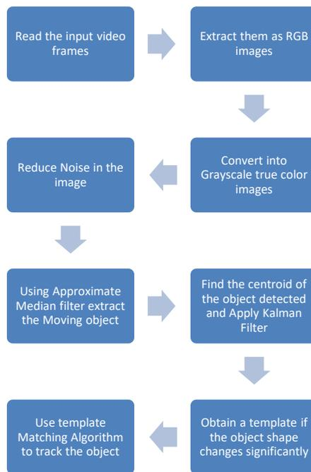
Figure 1 Block Diagram of the implementation and evaluation
