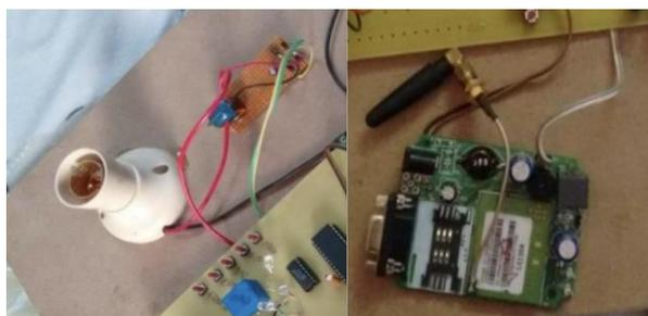
Load connection and GSM module
