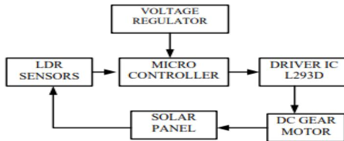
**Fig 3:**Block diagram of Single axis solar tracker
