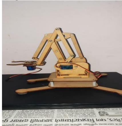
The above Figure (6) shows the hardware implementation of the proposed system. The Figure (7) shows the robotic arm used in the system. This robotic arm consists of 4 servo motors that allow free movement of the arm. We have successfully implemented the hardware implementation of the proposed system in real time.
