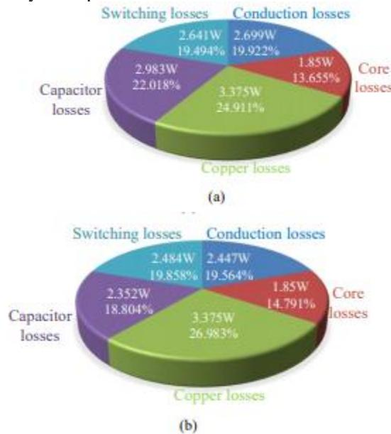
Fig. 22 Calculated power loss distributions for the experiment when  $U_{low}=40V$ ,  $U_{high}=300V$ , and  $P_n=300W$ . (a) In step-up mode. (b) In step-down mode.
