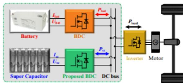
Fig. 19 Hybrid energy sources system of electric vehicles.
