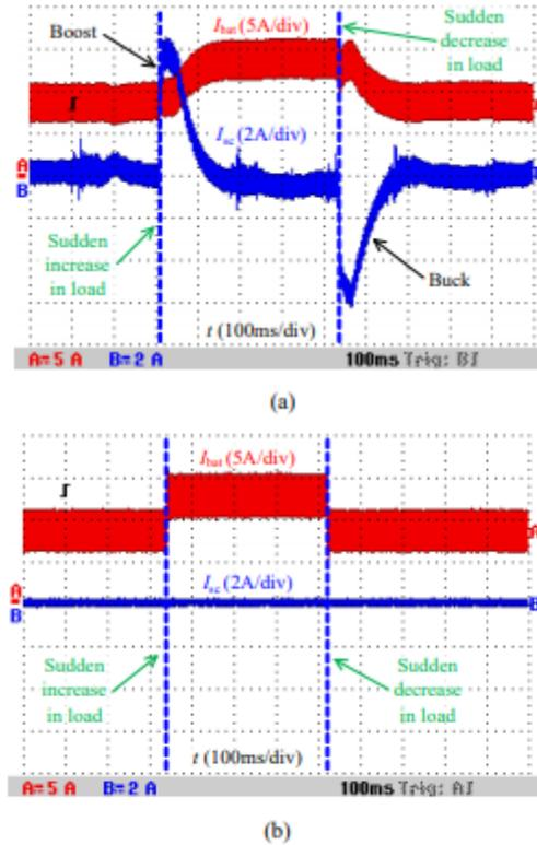
Fig. 20 Experimental results of bidirectional power flow control. (a) Super-capacitors are taken into operation. (b) Super-capacitors are not taken into operation.
