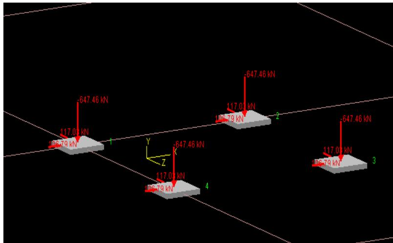
Fig no.9: Modeling of Isolated Footing in STAAD Foundation
