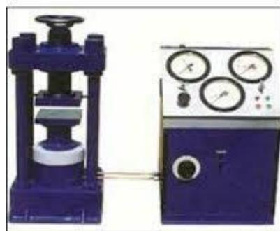
**Figure ; Compression test Equipment**
