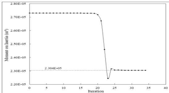
damaged member using the interior point method. The cross-sectional area and moment of inertia of the frame's damaged member are  $1.28 \times 10^{-2} \text{ m}^2$  and  $2.304 \times 10^{-5} \text{ m}^4$ . The identification results show that the final optimal value of A and I are identified and consistent with the frame's "as-is" condition.
