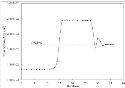
illustrates the plots of  $A_2$  and  $I_2$ , which is the cross-sectional areas and moment of inertia of damaged member, as a function of the iteration for case 2. The horizontal axis represents the iteration steps, while the vertical axis represents the values of  $A_2$  and  $I_2$ . The process of searching the cross-sectional area and moment of inertia of the damaged member using the interior point
