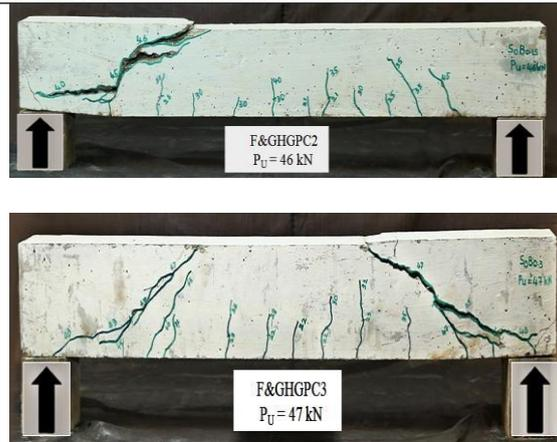
Fig. 4.1 Crack patterns showing shear failure of FHGPC specimens
