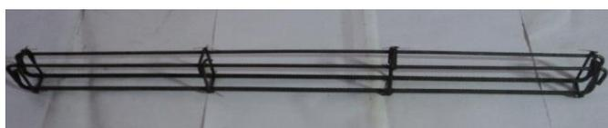
Fig. 3.5 Reinforcement cage
