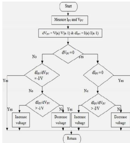
Fig. 3: Flowchart of Inc Con algorithm [Salas, 2006].
