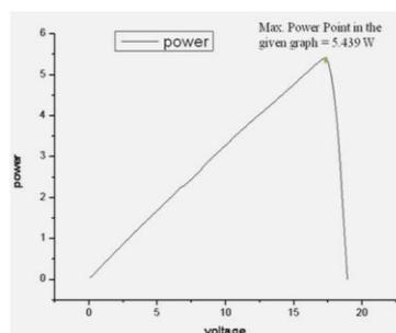
Fig. 1: I-V and P-V characteristics of PV module with MPP
