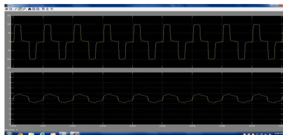
Fig 6: 3 level output voltage and current
