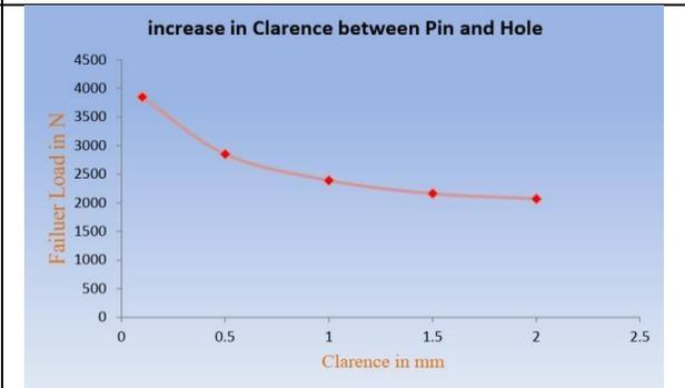
Figure 18: Failure Load for increase in Clarence between Pin and Hole
