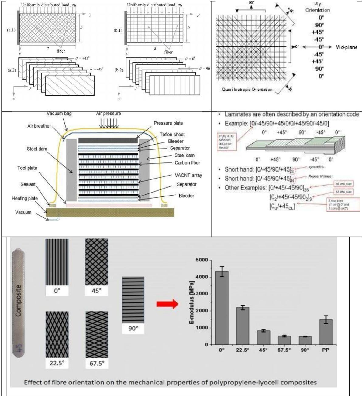
Figure 3: Ply orientation
