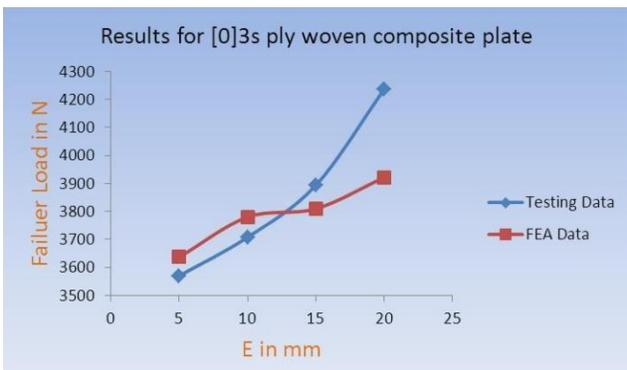
Figure 21: width = 20 mm, and depth ware vary from 5 to 20 with increment of 5 mm
