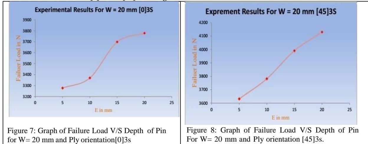
Figure 7: Graph of Failure Load V/S Depth of Pin for W= 20 mm and Ply orientation [0]3s
