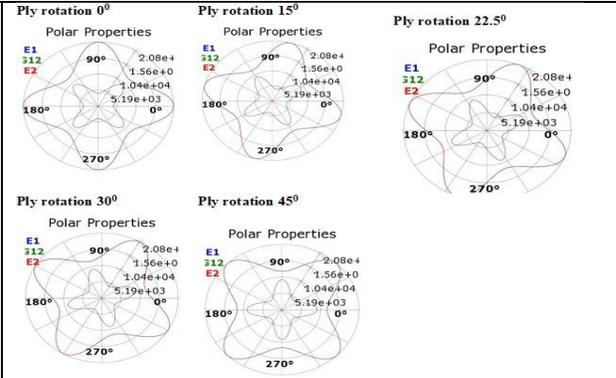
Figure 16: ply rotations form 0<sup>0</sup> to 45<sup>0</sup>
