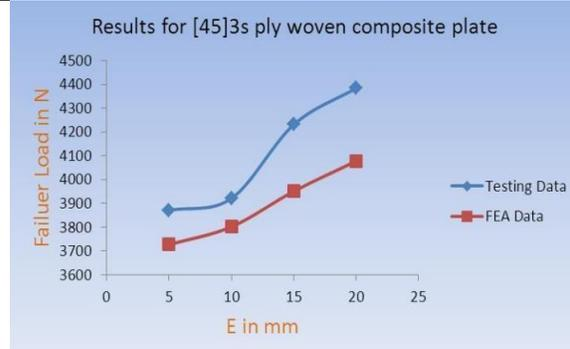
Figure 20: width = 20 mm, and depth ware vary from 5 to 20 with increment of 5 mm
