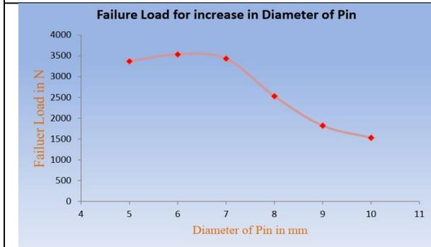
Figure 17: Failure Load for increase in Diameter of Pin
