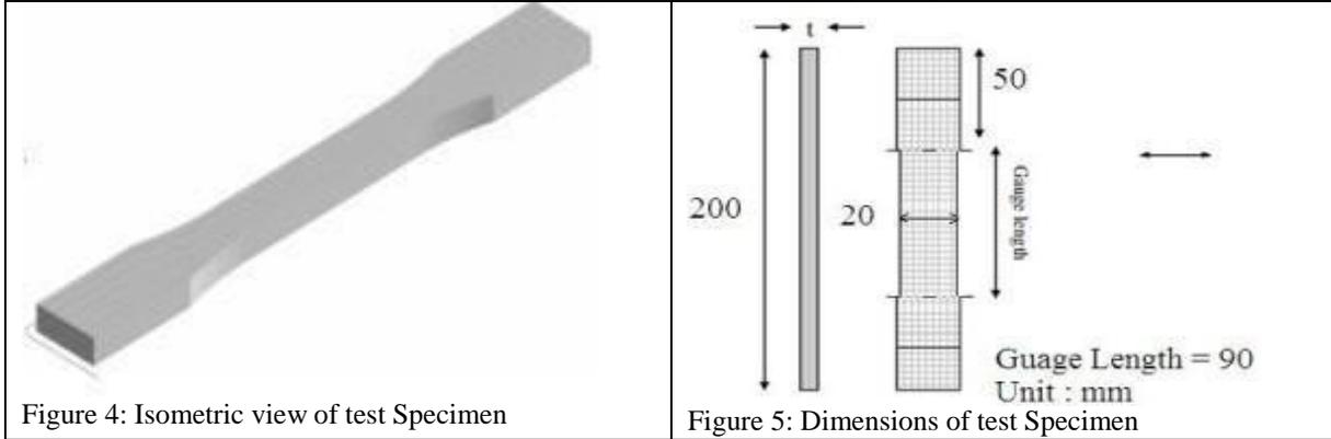
For geometrical variations total 16 specimens were cut in according to W/D and E/D ratio as shown in Table Below, and samples were named according to below configurations, with total length of 110 mm, 60 mm is working length for the specimen.
