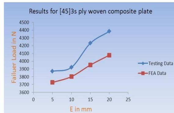
Figure 22: width = 20 mm, and depth ware vary from 5 to 20 with increment of 5 mm
