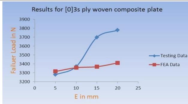
Figure 19: Width = 20 mm, and depth ware vary from 5 to 20 with increment of 5 mm
