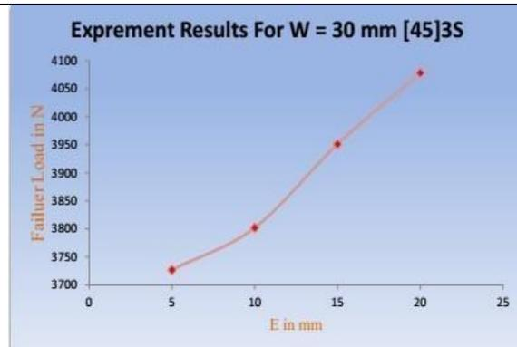
Figure 10: Graph of Failure Load V/S Depth of Pin for W= 30 mm and Ply orientation[45]3s
