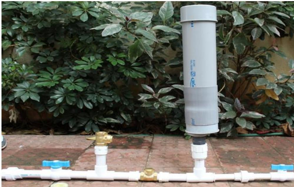
Fig. Completed assembly of the Ram Pump
