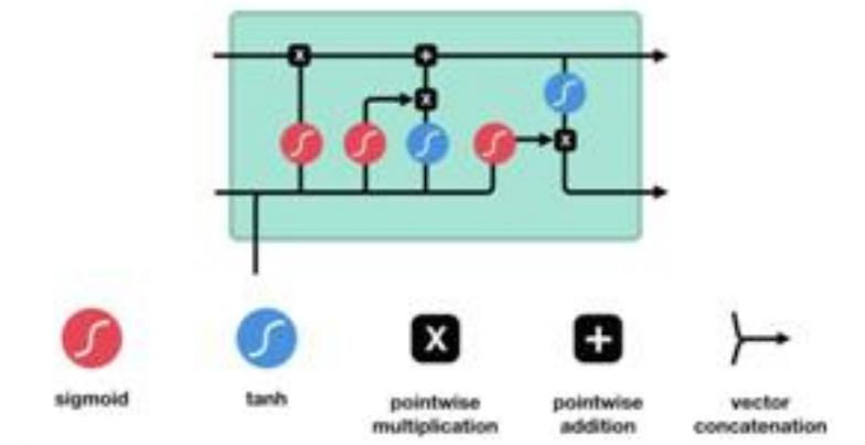
LSTM has a chain structure consisting of forums, neural networks and various memory blocks called cells. Information is maintained by cells and memory manipulations are done by gates. There are three gates –
