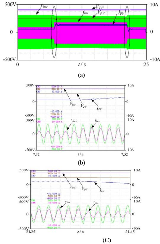
Fig.7 . Experimental results with load change. (a) Full view, (b) increasing load, and (c) decreasing load.
