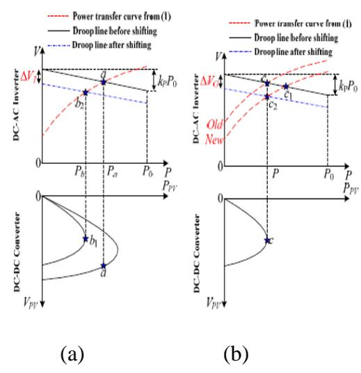
Fig. 5.  $P-V$  interactions during changes of (a) PV power and (b) grid voltage.
