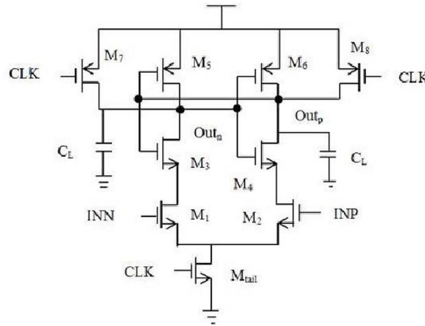
Figure 3: Fine Grain Single Tail Comparator
