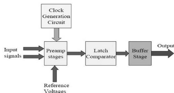
Figure 1: Comparator Architecture
