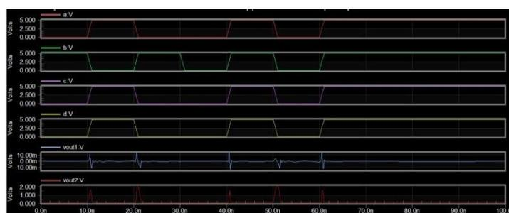
Simulation of Coarse Grain Double Tail Comparator
