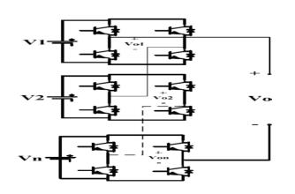
Fig 1. Cascaded H-bridge multilevel converter.
