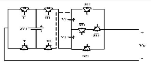
Fig 2. Proposed HCS topology under single basic unit.
