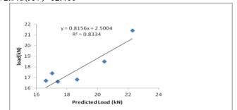
The statistical goodness of fit measures of the model, namely,  $R^2$  adj was 0.8334, the statistical measures were in the very good regime exemplifying that the model can be used to understand the total fracture load of the different asphalt mixtures.
