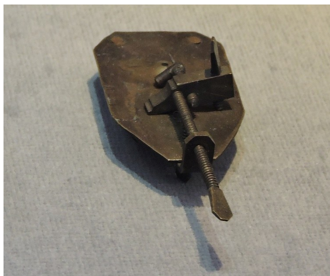
Figure 1. Replica of microscope that was used by Anthony van Leeuwenhook. Zeiss Museum of Optics, Jena. Credit: Stephanus H Coetzee.
