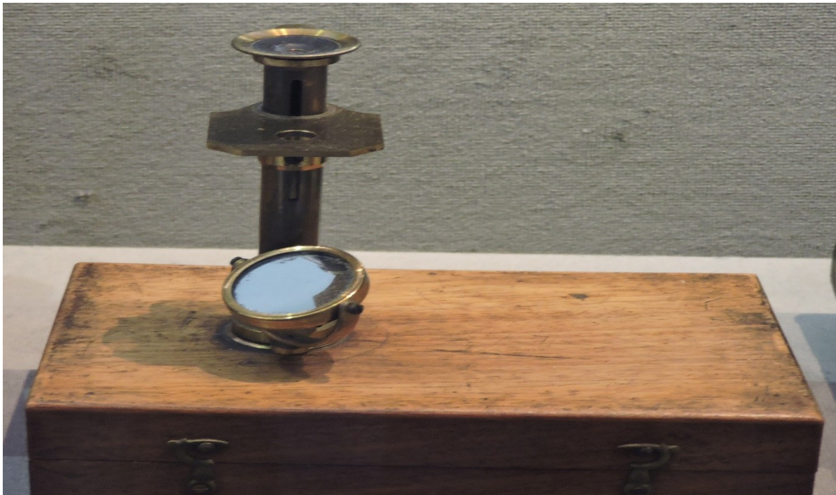
Figure 3. An early simple microscope with a fixed magnification. Zeiss Museum of Optics, Jena. Credit: Stephanus H Coetzee.
