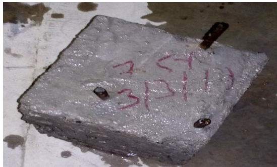
Fig.1 steel rods are inserted in concrete cubes
