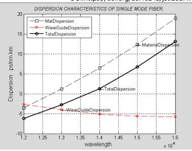
Figure 3 - Dispersion characteristics for singlemode fiber
