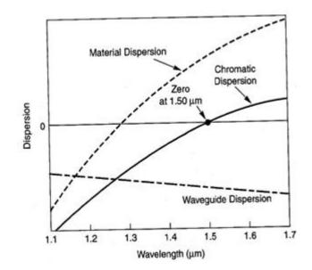
Figure 2- Combine waveguide and material dispersion.
