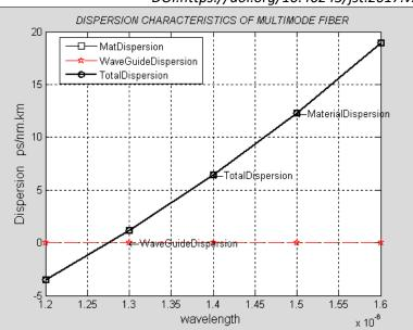
Figure 4- Dispersion characteristics for multimode fiber
