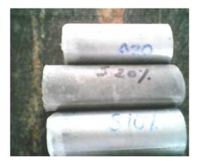
Motor through flexible link. Stirrer is used to stirrer the molten metal in semi-solid state. The screw operator lifting is used to bring the stirrer in contac Figure 3.2 Fabricated materialin composite material. The melt is maintaining at a particular temperature, which is depends on matrix material for one hour. Vortex is creating using a mechanical stirrer. Preheated particle reinforcement will add to the melt during stirring. Stirring will be carried out for 5 min at 180 rpm for all samples.
