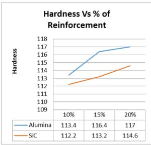
Figure 4.2.1 shows that increase in percentage of reinforcement tends to increase in hardness, here alumina reinforced composite processes higher hardness value compare to Silicon carbide reinforced composite which is suitable for the application.
