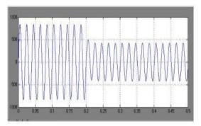
Figure4. Load voltage with sag conditions
