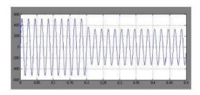
Figure 12.Load voltage with sag conditions
