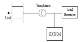
Figure 1. Voltage Fluctuation Mitigation with STATCOM
