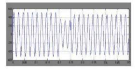
Figure 8.Load voltage with sag conditions
