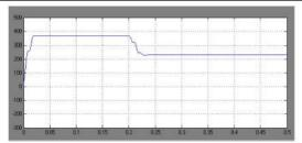
Figure 18.RMS Load voltage with sag condition
