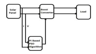
Figure 4: Block diagram
