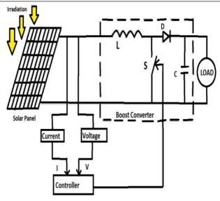
Figure 3: Boost converter with MPPT
