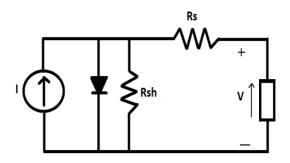
Figure 1: Equivalent Circuit of solar cell
