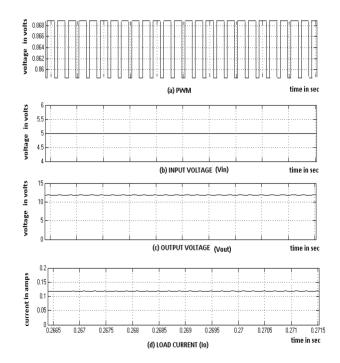
Figure 9: Simulation results for boost converter with PI controller (a)PWM , (b)Input Voltage, (c)Output Voltage and(d)Load Current
