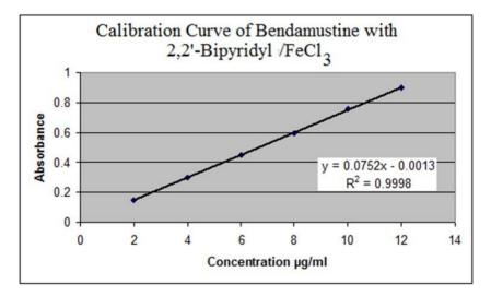
Figure 1: Calibration Curve of Bendamustine hydrochloride
