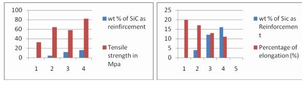
Tensile strength of sic Reinforcement
